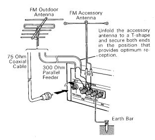
**CAUTION:** Never make a connection to a gas pipe because it can cause fire hazard.
