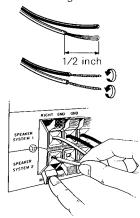
**CAUTION:** Two speaker systems can be connected to this unit. The minimum speaker impedance should be 8 Ohm when only one speaker system is connected. When two speaker systems are connected, care should be taken that net impedance does not become less than 8 Ohm.
